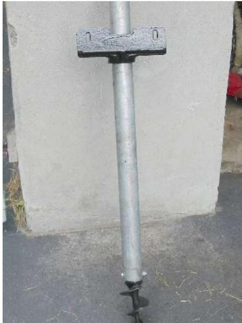
Figure 7 – Pipe with auger and dock fitting attached.
