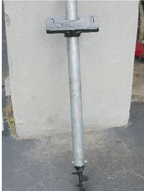
Figure 7 – Pipe with auger and dock fitting attached.
